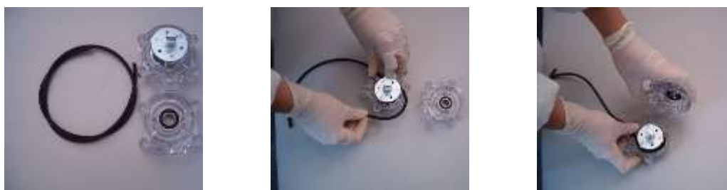
Figure 7.1: Pump tubing replacement.
