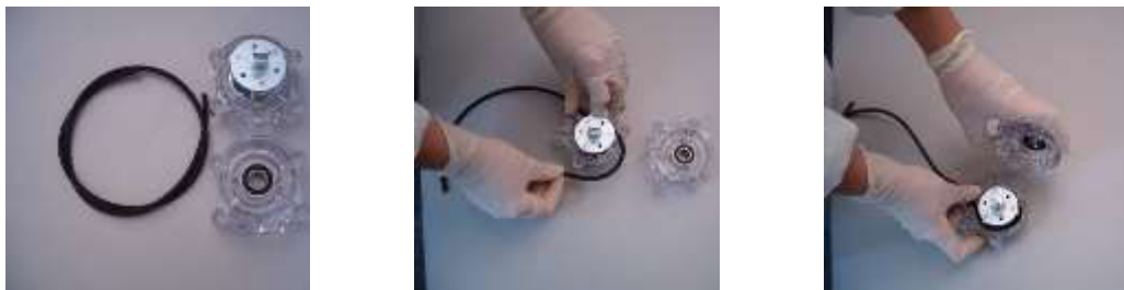
Figure 7.1: Pump tubing replacement.
