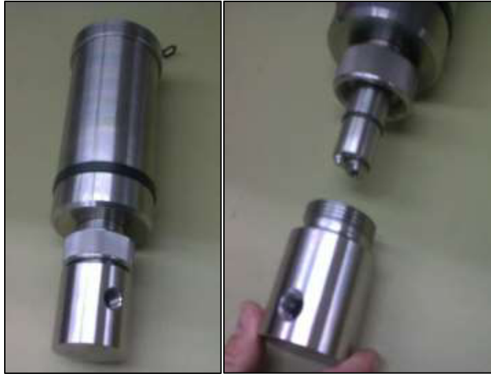
Figure 3.3: Fitting the sensor into the flowcell.
