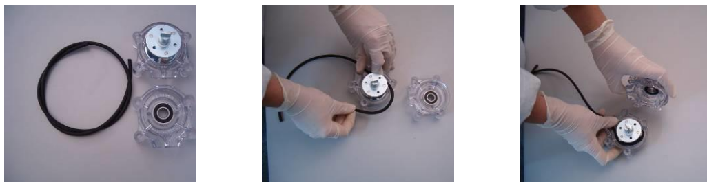
Figure 7.1: Pump tubing replacement.
