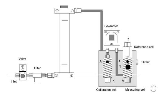
Arrangement of the wall mounted instrument (optional Salting Cell shown)
