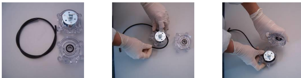
Figure 7.1: Pump tubing replacement.
