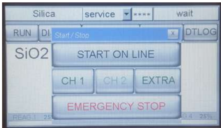
Figure 5.3: User interface after pressing the RUN Menu.
