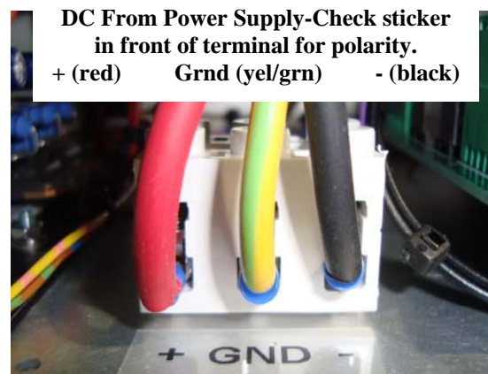
Figure 2.7 – Power Supply Terminal
