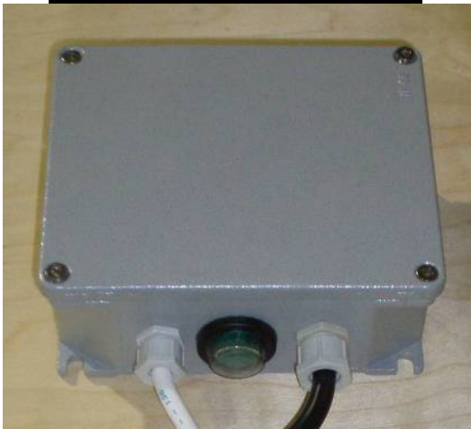
Figure 2.5 - User Junction Box
