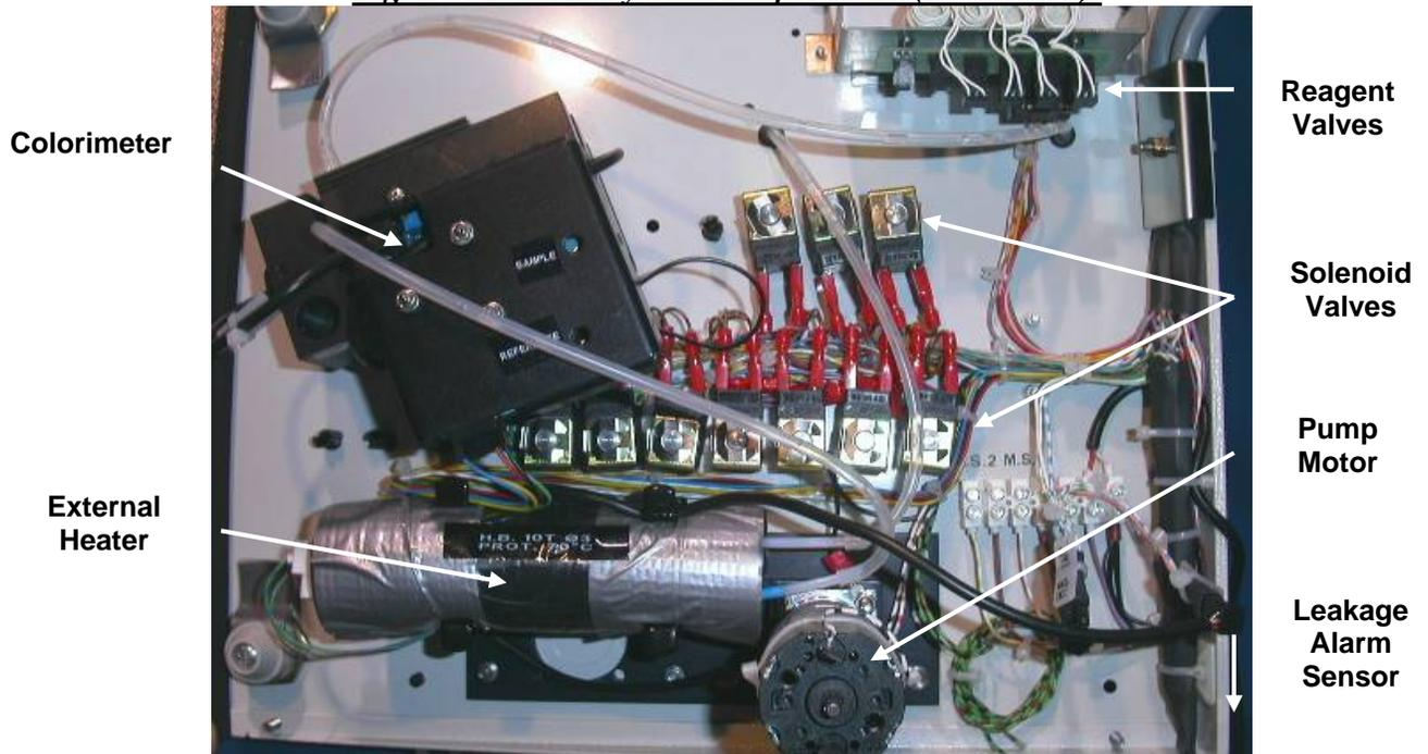
3 Liquid Handling Section-Analytical Compartment
