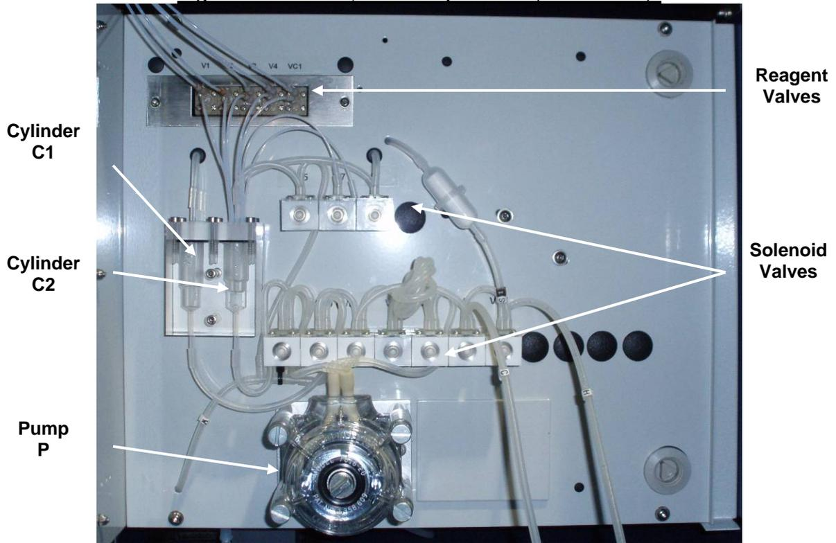
**Figure 3.2 — Analytical Compartment (Back View):**
