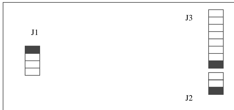
Figure 9. Pre-amplifier layout. Pin 1 of all the connectors is shown in black.
