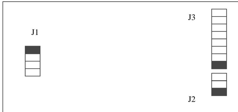
**Figure 7.** Pre-amplifier layout. Pin 1 of all the connectors is shown in black.
