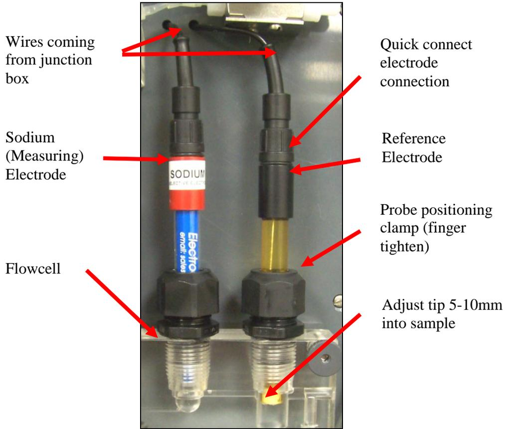
The Gel filled reference electrode has an inner element consisting of a gel solution which does NOT require electrolyte refilling.
