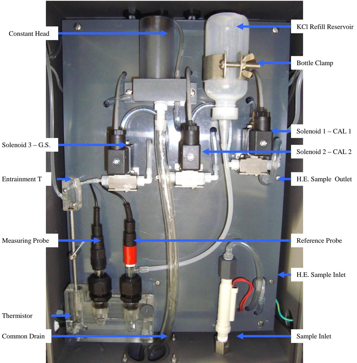
**Figure 6. The wet section layout and connections.**
