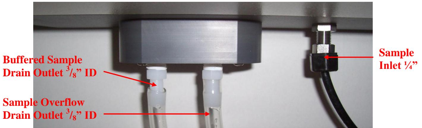
**Figure 5.** The bottom of the wet section case, with the sample inlet and drain connections shown.
