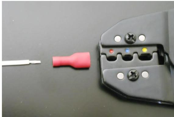
**Figure 2:** Select the appropriate terminal based on the wire gauge used. Red-colored terminals handle 22-18AWG; blue terminals are for 16-14AWG and yellow are for 12-10AWG. Note the corresponding color dots on the crimp tool die set. Match the terminal to the position on the die. Do not over-crimp by using a smaller die position for the terminal – you will damage the wire strands and wind up with a weak connection.
