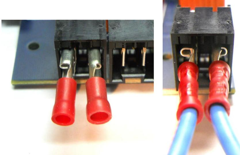
**Figure 4A:** Only partially shrouded terminals will fit onto the Analog Board's connectors. An assortment of suitable connectors and a crimp tool is supplied in Waltron's Terminal Kit, p/n 907-0000-00. Note that the orientation of the terminals is important to maintain maximum electrical separation. Position the connectors facing in the directions shown before fully inserting.
