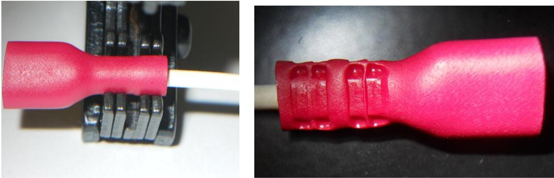
**Figure 3A:** Position the terminal in the die, as shown at the left. It is important to have the terminal positioned so that the connector end of the terminal is even with the jaw and the crimp part of the terminal mates correctly with the crimp tool die.
