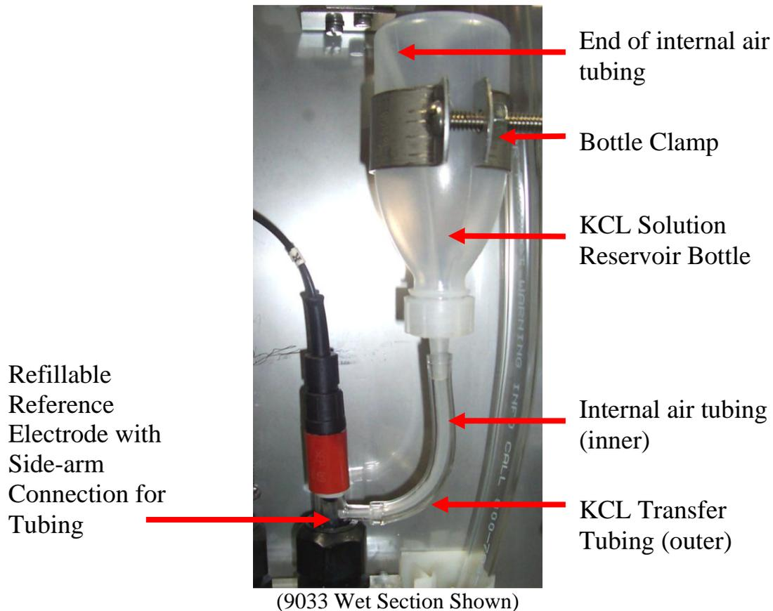
Directions for installing and using the KCl refill system:
