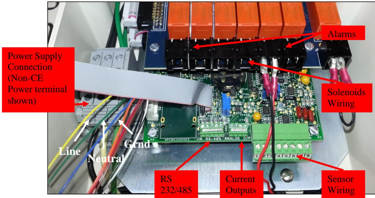
**Figure 10.** Location of the terminal block connections in the transmitter unit.
