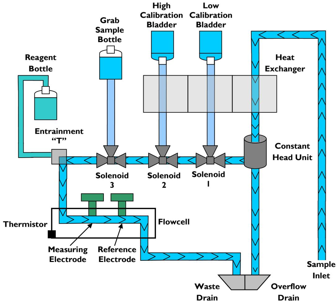
**Figure 12.** Sample flow during normal operation.
