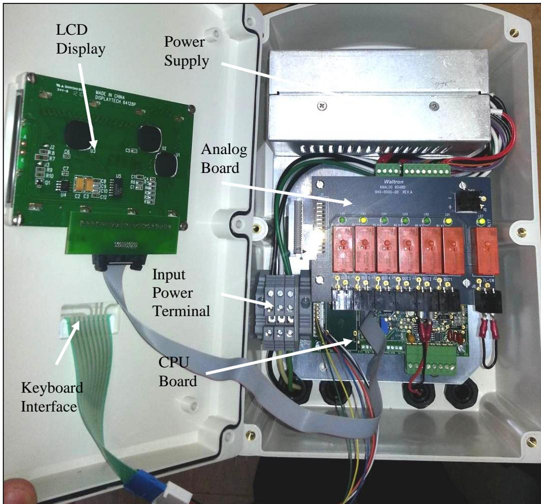
**Figure 9.** The layout and components of the transmitter case.
