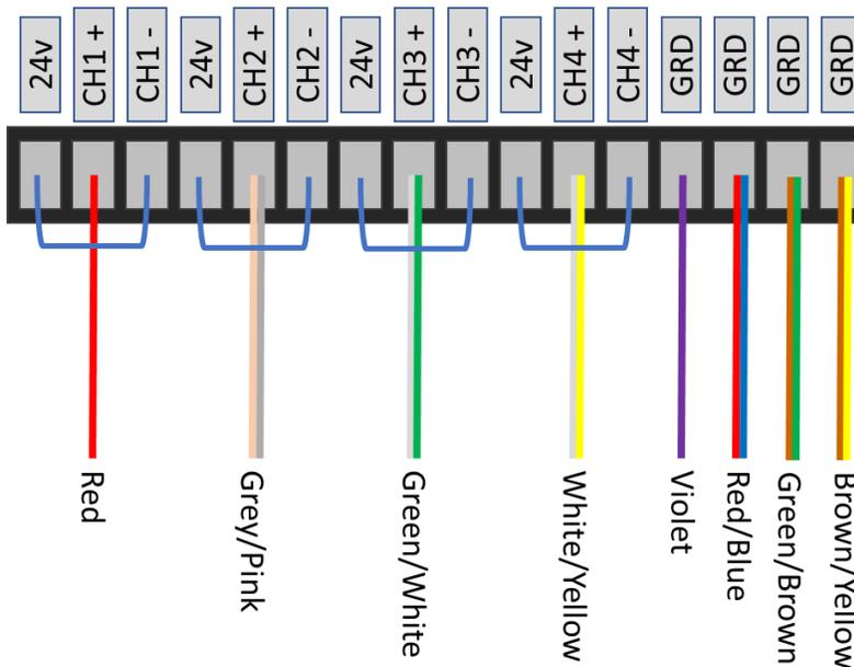
Figure 3.10: Powered Relay Configuration of J6; All Relays.
