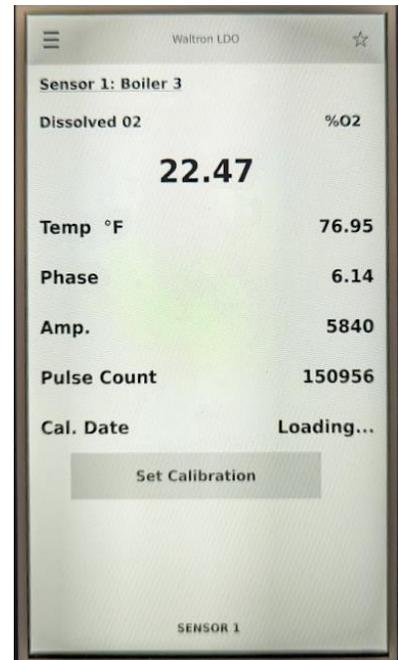
10. Allow the sensor to rinse down for approximately 15 minutes. Before proceeding, verify that the actual O<sub>2</sub> value is stable. For a 0% calibration, the phase value should be between 65 - 68 and stable at its highest point.
