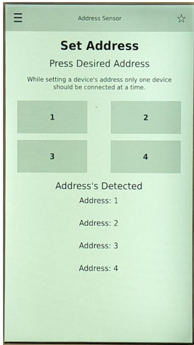
Note: Should a sensor not have an established address, the field will remain blank. Tapping an address will write to the new sensor, but will require that the transmitter conduct a soft restart. This will happen automatically.
