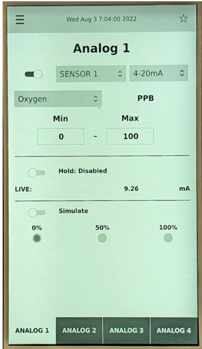
The bottom of the screen will appear with the available output channels and allows for easy switching between outputs in this screen.
