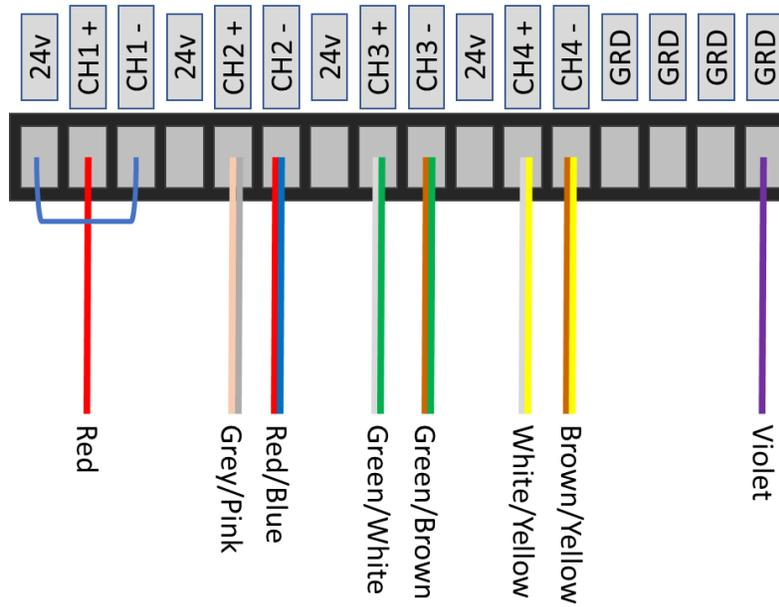
Figure 3.10: Powered Relay Configuration of J6; Relay #1 only.
