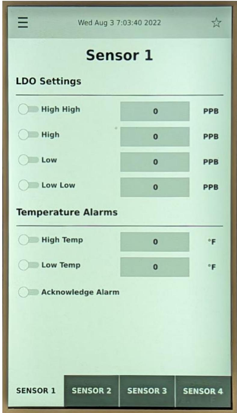
The bottom of the screen will appear with the addresses of the sensors detected and allow for easy switching between sensors in this screen.
