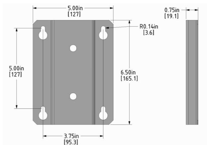
Figure 3.2: Dimensions of the 9165 sensor mounting bracket.
