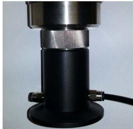
5. Connect calibration gas to the inlet of the calibration beaker.
