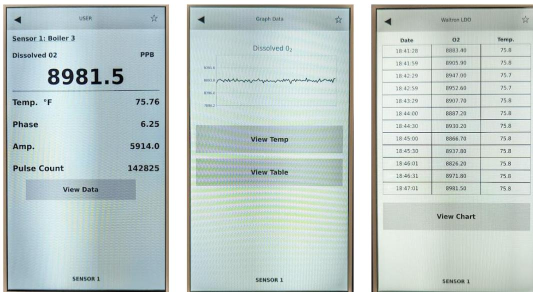
Tapping on view data will bring up a trendline plot of the trailing 100 readings. This can be toggled between Oxygen and Temperature by pressing View Temp or View O2.
