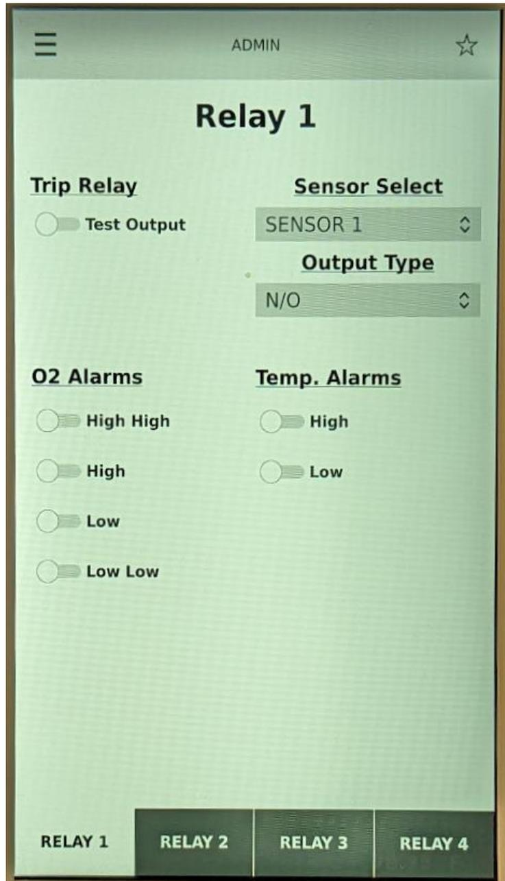
The bottom of the screen will appear with the available relay channels and allows for easy switching between outputs in this screen.
