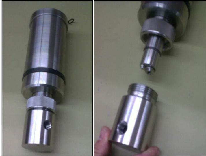
**Figure 3.3: Fitting the sensor into the flowcell.**
