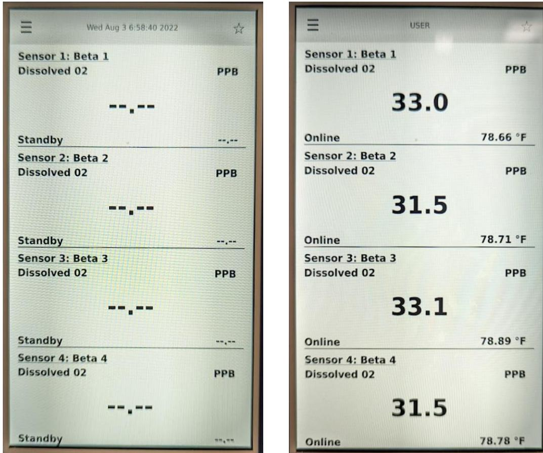
**Figure 4.2: Left: Main screen with the analyzer in stand-by mode, Right: Main Screen in Online Mode**
