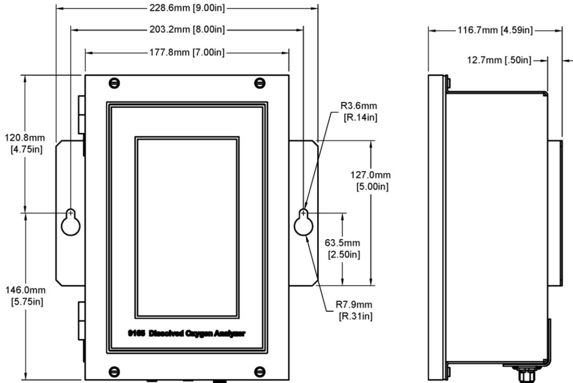
Figure 3.1: Dimensions of the 9165 transmitter for wall mounting.
