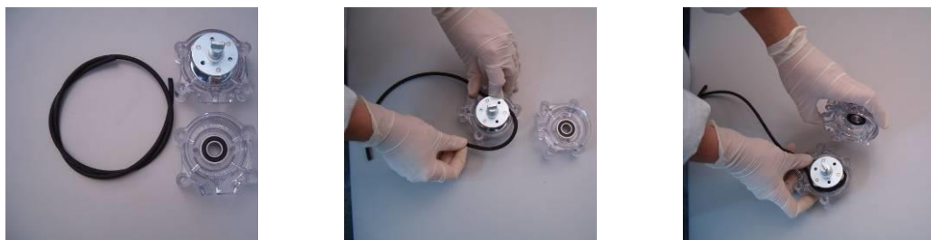
Figure 7.1: Pump tubing replacement.
