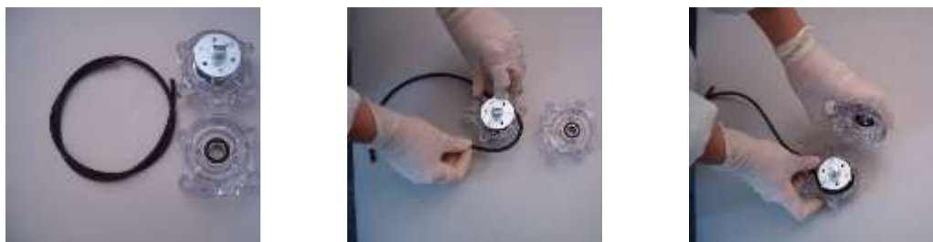
Figure 7.1: Pump tubing replacement.
