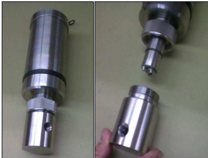
Figure 3.3: Fitting the sensor into the flowcell.
