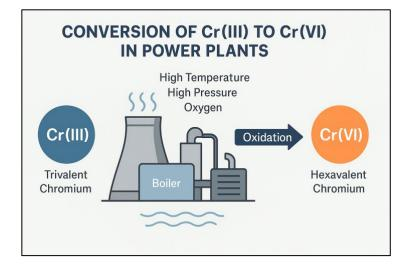
In power plants, particularly those running steam turbines, the conditions inside boilers and cooling systems are intense—high pressure, high heat, and plenty of oxygen. Combine this with the chromium alloys in pipes and machinery, and suddenly you've got the perfect environment for Cr(VI) formation. Add in the historical use of chromate-based corrosion inhibitors, and the problem multiplies.
