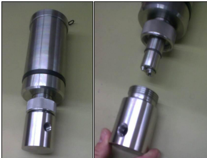
Figure 3.3: Fitting the sensor into the flowcell.
