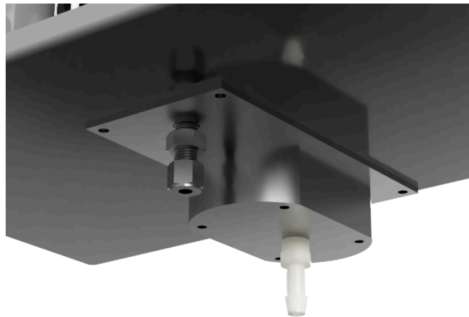
Figure 5. The bottom of the wet section case, with the sample inlet and drain connections shown.
